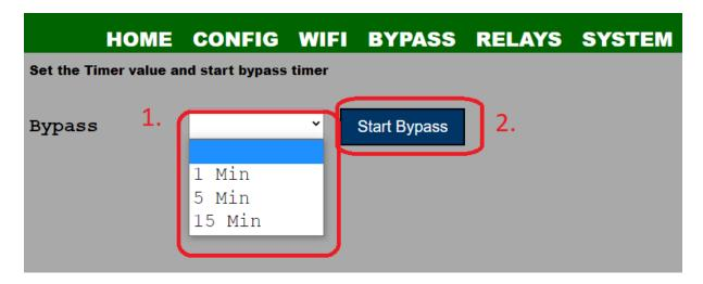
The Bypass button is not permeant due to safety reasons. You can choose 4 settings for bypass to help move the crane if it is stuck or if you haven't finished installing the system yet and need to move the crane.
