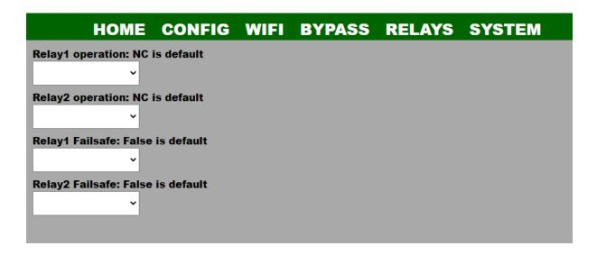
To Change the operation of the relay Pick the relay you want to swap the contact via the drop down menu and change it from NC to NO
