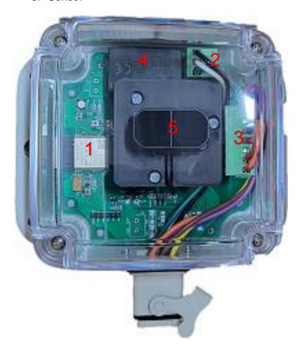
The LAC-12 has a 12 Meter (36ft) Range with 2 relay setpoints The relay setpoints are adjustable via the LAC-12 Webapp and real time distance is available in the webapp as well as the relay status of each relay.
