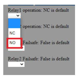
Now the relay will not close on startup and will turn on when the setpoint has been reached.
